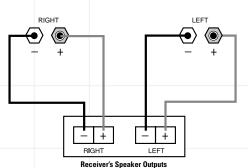
surround-sound systems, connecting all of the speakers in your system with the correct polarity remains equally important in order to preserve the proper ambience and directionality of the program material. To use the binding-post speaker terminals, unscrew the collar until
